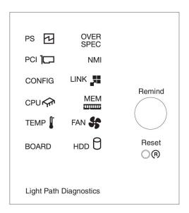
• **Remind button:** This button places the system-error LED/check log LED on the front panel into Remind mode. In Remind mode, the system-error LED flashes once every 2 seconds until the problem is corrected, the server is restarted, or a new problem occurs.
