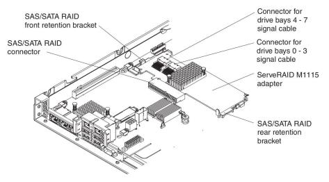
• ServeRAID M5110 adapter: Take the signal cable that is attached to the drive backplane for drive bays 4 through 7 and connect it to the ServeRAID adapter connector for drive bays 4 through 7 (port 1). Connect the other signal cable that is attached to the drive backplane for drive bays 0 through 3 and connect it to the other connector (port 0) on the adapter.
