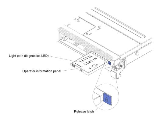
The following illustration shows the LEDs and controls on the light path diagnostics panel.
