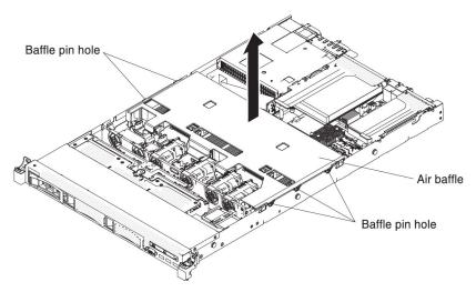
5. Remove the air baffle from the server and set it aside.
