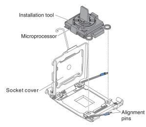
d. Twist the handle on the microprocessor tool counterclockwise to insert the microprocessor into the socket. The microprocessor is keyed to ensure that the microprocessor is installed correctly. The microprocessor rests flush on the socket only if properly installed.
