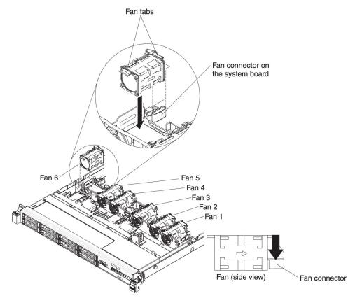
5. Orient the fan over the fan slot in the fan assembly bracket so that the fan connector aligns with the connector on the system board.
