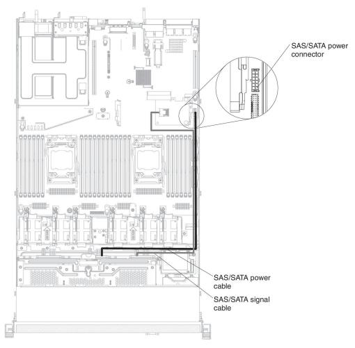
The following illustration shows the internal routing and connectors for the 3.5-inch simple-swap hard disk drives SATA signal and power cables.
