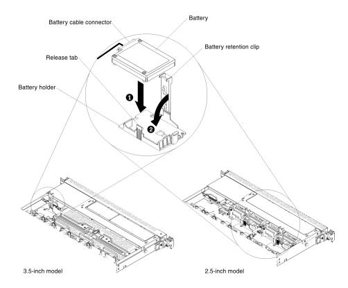
**Note:** The positioning of the remote battery depends on the type of the remote batteries that you install.
