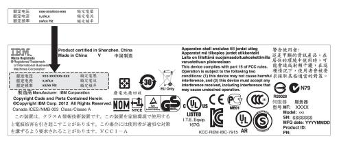
10. If you are adding a power supply to the server, attach the redundant power information label that comes with this option on the server cover near the power supplies.
