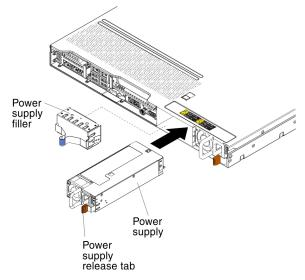
4. Grasp the handle on the rear of the power supply and slide the power supply forward into the power-supply bay until it clicks. Make sure that the power supply connects firmly into the power-supply connector.
