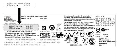
13. If you are adding a power supply to the server, attach the redundant power information label that comes with this option on the server cover near the power supplies.
