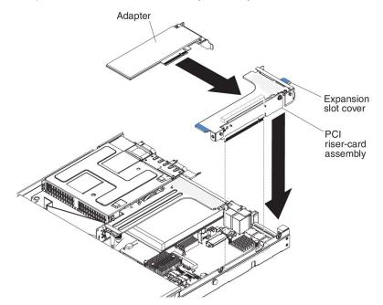
**Attention:** When you install an adapter, make sure that the adapter is correctly seated in the riser-card assembly and that the riser-card assembly is securely seated in the riser-card connector on the system board before you turn on the server. An incorrectly seated adapter might cause damage to the system board, the riser-card assembly, or the adapter.
