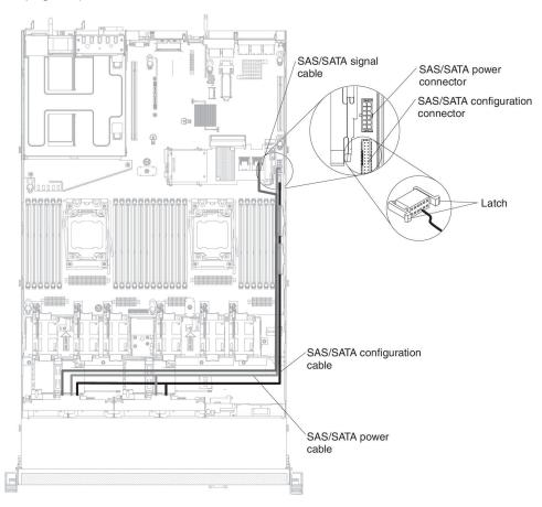
9. Connect the signal cables to the SAS/SATA adapter:
