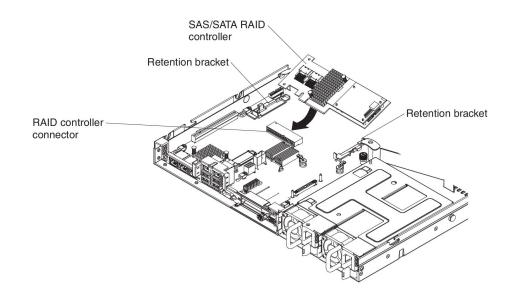
b. Insert the SAS/SATA adapter into the PCI riser cards. (see "Installing an adapter" on page 67).
