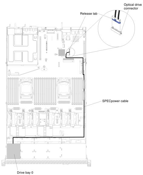
The following illustration shows the internal routing and connectors for the server models with one 2.5-inch simple-swap hard disk drives.
