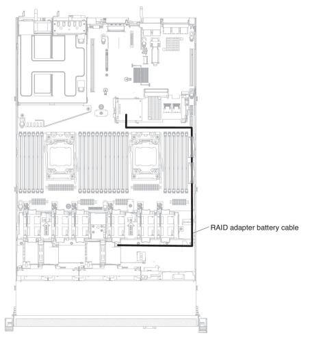
**Attention:** Make sure that the cable is not pinched and does not cover any connectors or obstruct any components on the system board.
