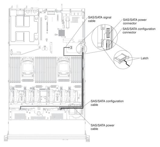
The following illustration shows the internal routing and connectors for the SAS/SATA signal, power and configuration cables with the SAS/SATA adapter installed.
