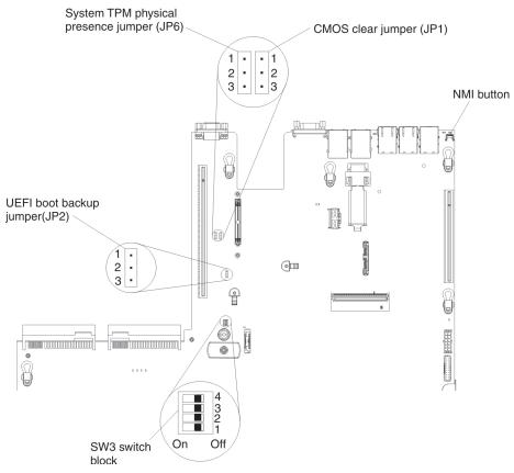
**Attention:** Before you change any switch settings or move any jumpers, turn off the server; then, disconnect all power cords and external cables. See the safety information that begins on page vii. Do not change settings or move jumpers on any system-board switch or jumper block that is not shown in this document.
