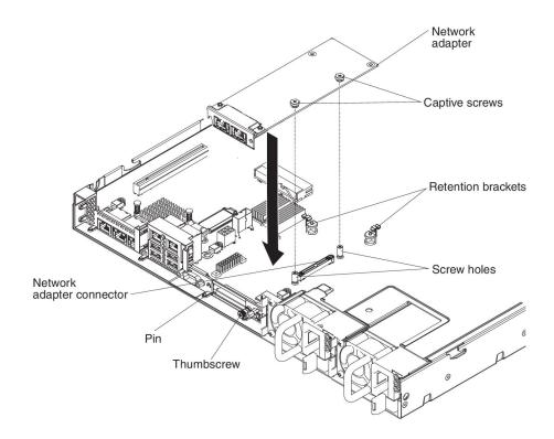
8. Press the adapter firmly until the pin, standoffs, and retention brackets engage the adapter. Make sure the adapter is securely seated on the connector on the system board.
