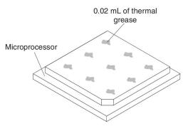
5. Use the thermal-grease syringe to place 9 uniformly spaced dots of 0.02 mL each on the top of the microprocessor. The outermost dots must be within approximately 5 mm of the edge of the microprocessor; this is to ensure uniform distribution of the grease.
