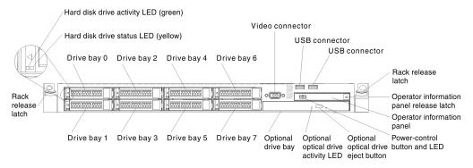
The following illustration shows the controls, LEDs, and connectors on the front of the 3.5-inch hard disk drive server model.
