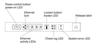
• **Power-control button and power-on LED:** Press this button to turn the server on and off manually. The states of the power-on LED are as follows:
