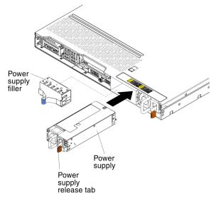
6. Grasp the handle on the rear of the power supply and slide the power supply forward into the power-supply bay until it clicks. Make sure that the power supply connects firmly into the power-supply connector.
