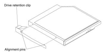
9. Align the drive in the drive bay and slide the drive into the optical drive bay until the drive clicks into place.
