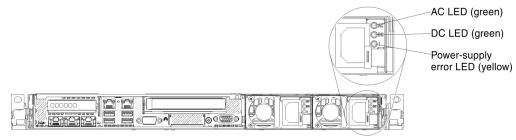
The following table describes the problems that are indicated by various combinations of the power-supply LEDs on an ac power supply and suggested actions to correct the detected problems.
